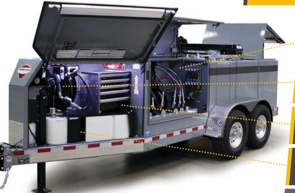
**VERSATILE.** Customize for up to eight systems of oils, coolant, diesel, and used oil reclaim. DEF and grease systems as well.
